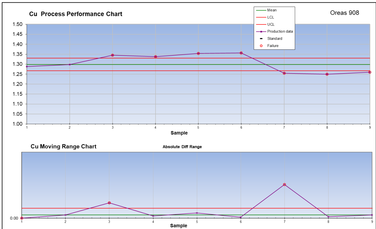
Figure 8-26: Santa Cruz Deposit, OREAS 908 standard total Cu (g/t), assayed at American Assay Laboratories
