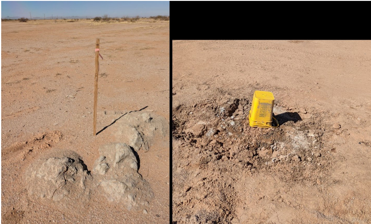
Figure 9-2: Collars for historic diamond drill holes CG-091 and CG-030
