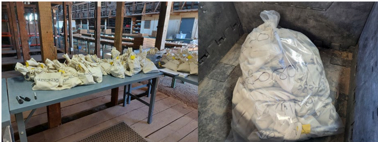
Figure 8-3: (Left) samples placed in burlap and inner plastic bags labeled with sample numbers; (Right) sample batches placed in large plastic bags and bins for shipping to lab
