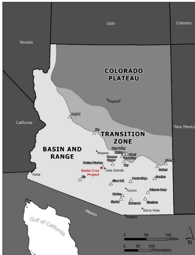
Figure 6-1: Regional geology of the Southwestern Porphyry Copper Belt and the Cu porphyry deposits in the area around the Santa Cruz Project.
