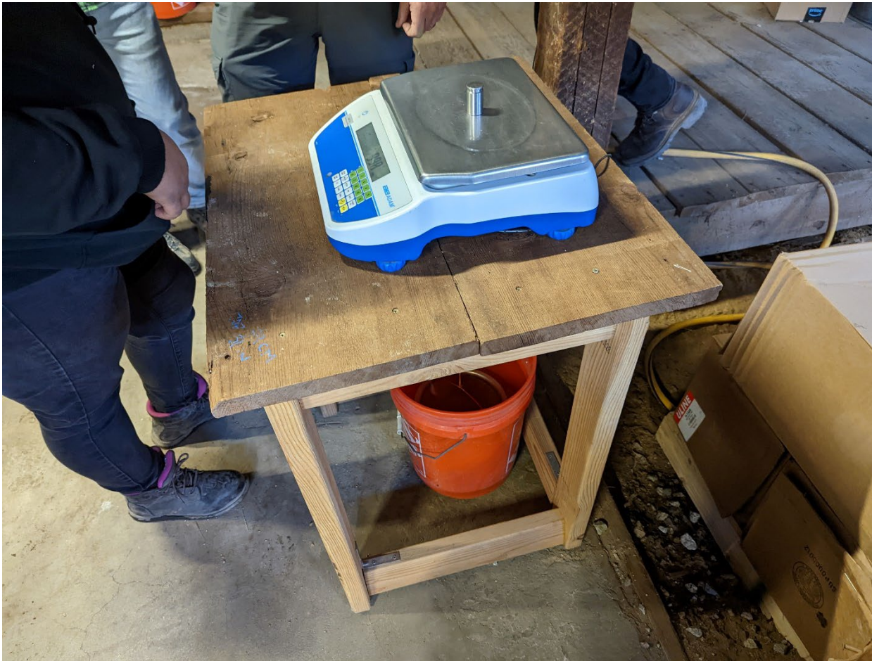
Figure 9-6 Specific gravity measuring station within core logging facility.
