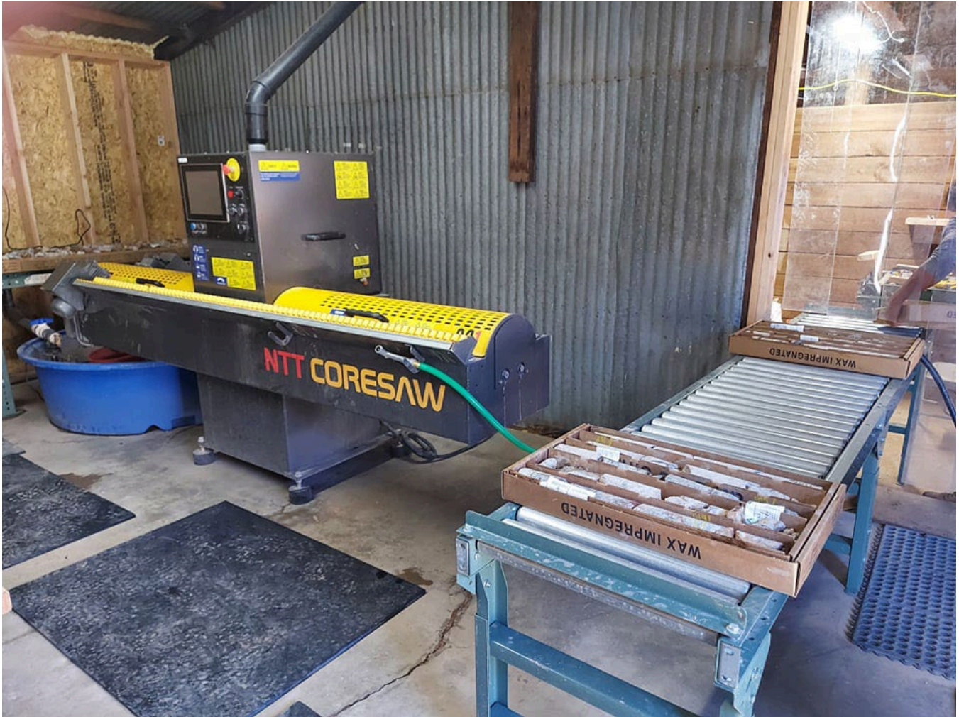
Figure 8-1: NTT diamond bladed automatic core saw used for cutting diamond drill core for sampling.
