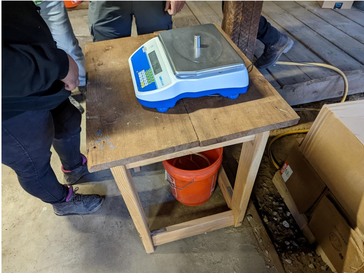
Figure 12-6 Specific gravity measuring station within core logging facility.
