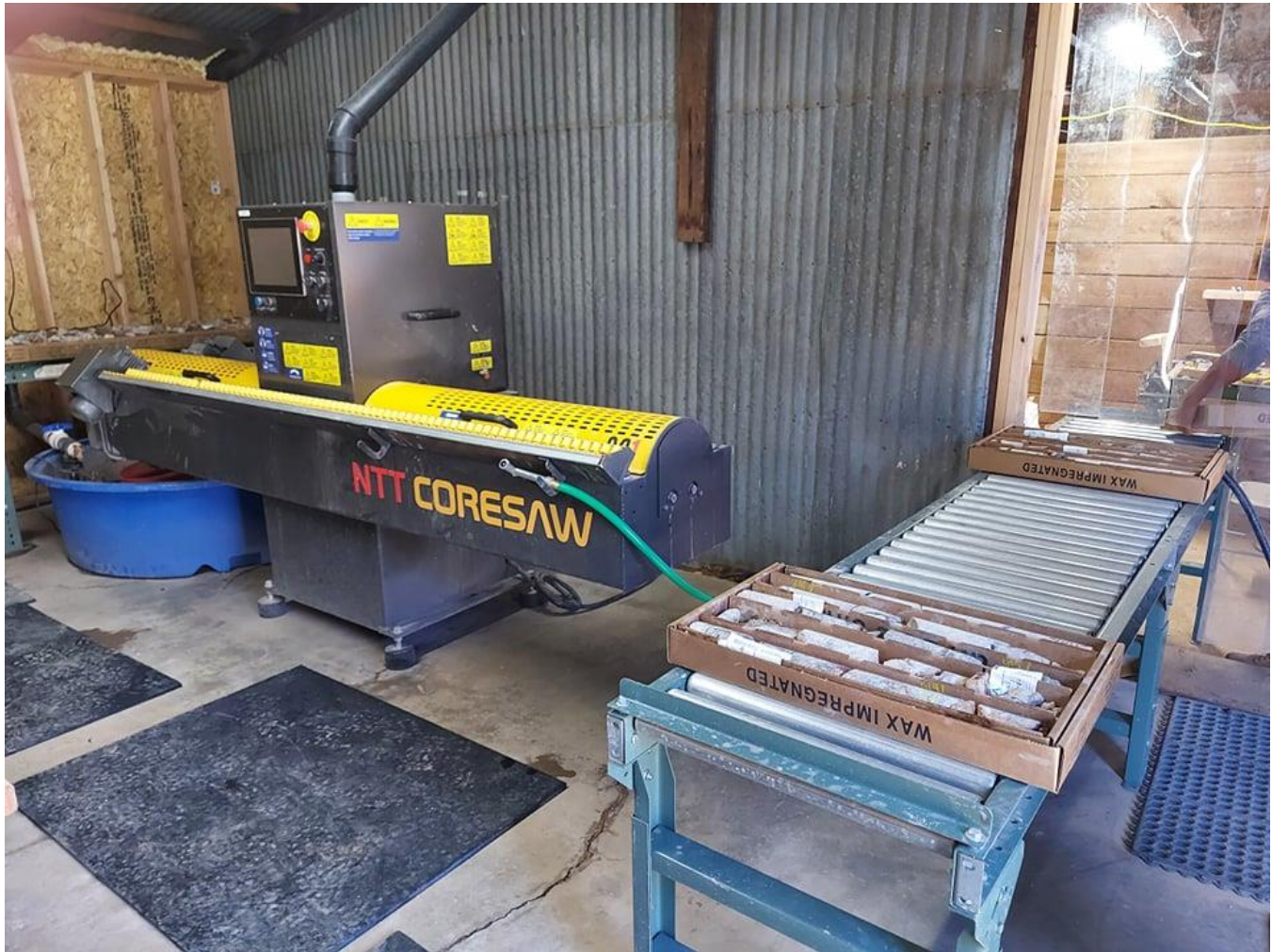
Figure 11-1: NTT diamond bladed automatic core saw used for cutting diamond drill core for sampling.
