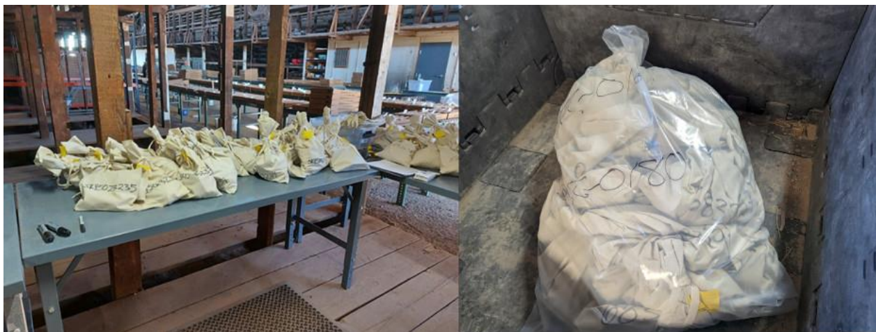
Figure 11-3: (Left) samples placed in burlap and inner plastic bags labeled with sample numbers; (Right) sample batches placed in large plastic bags and bins for shipping to lab
