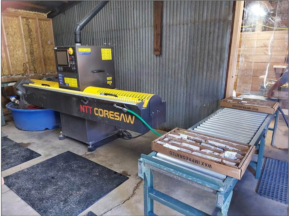
Figure 8-1: NTT Diamond Bladed Automatic Core Saw used for Cutting Diamond Drill Core for Sampling
