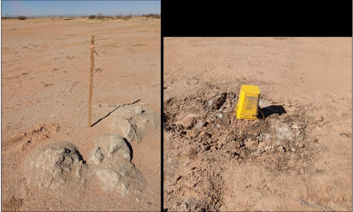
Figure 12-2: Collars for Historic Diamond Drillholes CG-091 and CG-030
